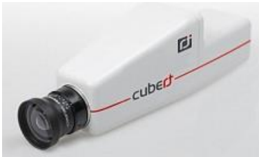
Cubert S185 450-950nm, 125 channels weight 470g, frame - 1 / 1000sec, for UAVs, starting - 840g
